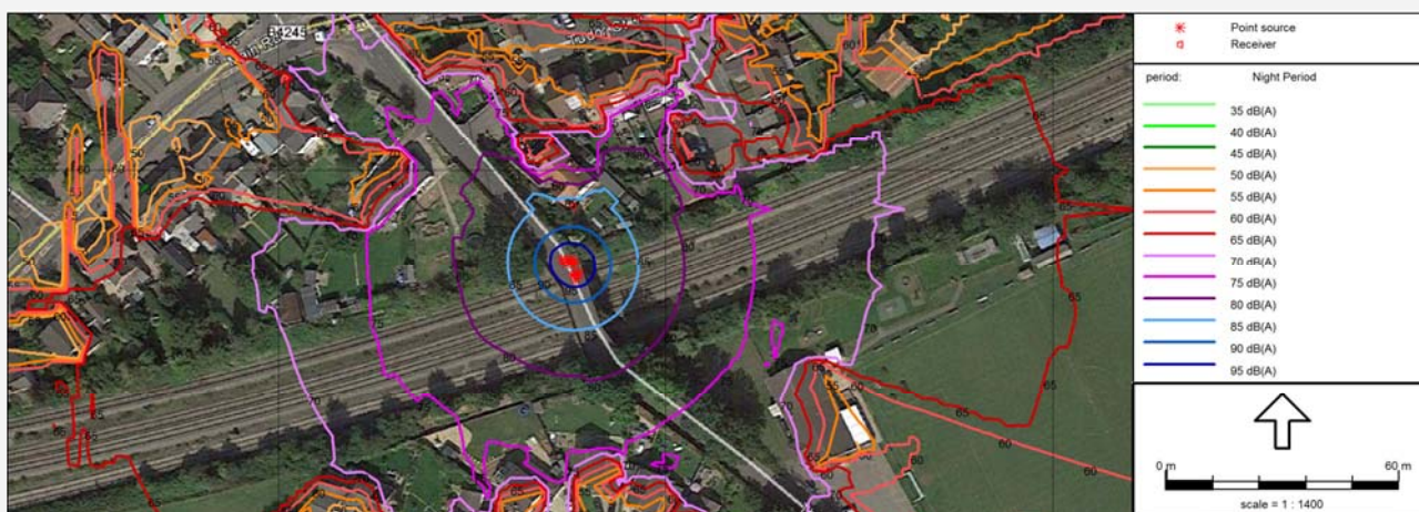
Noise Contour Map showing predicted noise levels during part of a bridge replacement project
